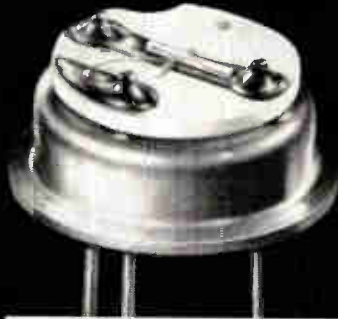
Greatly magnified photo of silicon transistor showing Fixed Bed Construction. All parts are firmly fastened, with no suspended parts except wire lead. Transistor reacts as a solid block in resisting shock and vibration. Power dissipation is inherently higher.
