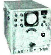
Model TSA-W Wide Dispersion Spectrum Analyzer — 100 kc to 70 mc dispersion. 7 kc and 50 kc resolution. Logarithmic amplitude display. 5 sensitive plug in tuning units.
