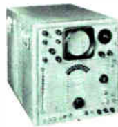
Model TSA-S Combination Synchroscope-Spectrum Analyzer — Displays pulse waveform or frequency spectrum. 5 kc to 5 mc adjustable bandwidth, 400 kc to 25 mc dispersion. 5 sensitive plug-in tuning units.
