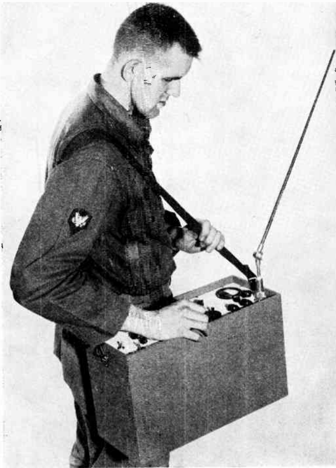
Fig. 13—Radio interference-measuring set AN/PRM; (mock-up). (Lab. Design.-Constr.) Frequency range: 75-500 mc. Overall \frac{3}{4} view, showing personnel demonstrating operation of model.
