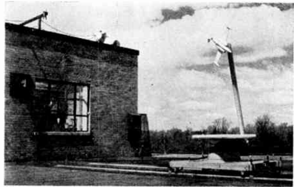
Fig. 20—A scale-model aircraft and antenna mounted for pattern measurements (National Research Council of Canada photograph).
