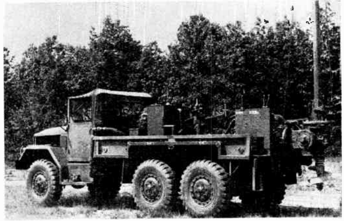
Fig. 15—Auger, earth, truck-mounted LC-245(XC-2)/M (Devel. model). Installed in cargo space of truck, 2\frac{1}{2} ton, 6X6, cargo M34. Manufactured by Highway Trailer Co. Roadside rear \frac{3}{4} view, showing rack bar and guide tube in raised position, ready for digging.
