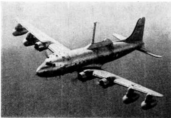
Fig. 1—The flying laboratory. The nacelles under the wings contain steerable 47" dish radar antennas, three with variable polarization. The 15' retractable mast carries a Texas refractometer, the NRL ultraviolet humidimeter and other meteorological probes of slower response.
