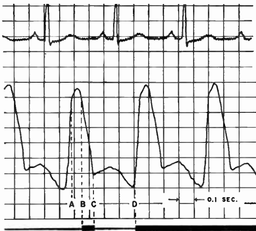
Fig. 4—Reproduction of Twin-Viso recording showing ECG tracing, aortic pressure wave, and stylus marking to indicate series of operations. A-B, injection delay; B-C, duration of injection; A-D, X-ray delay.
