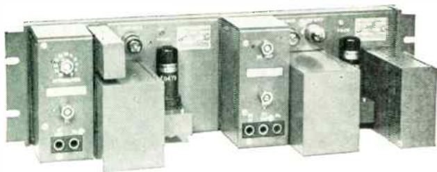
A send and a receive panel require 5 1/4" of mounting space on a standard 19" rack
