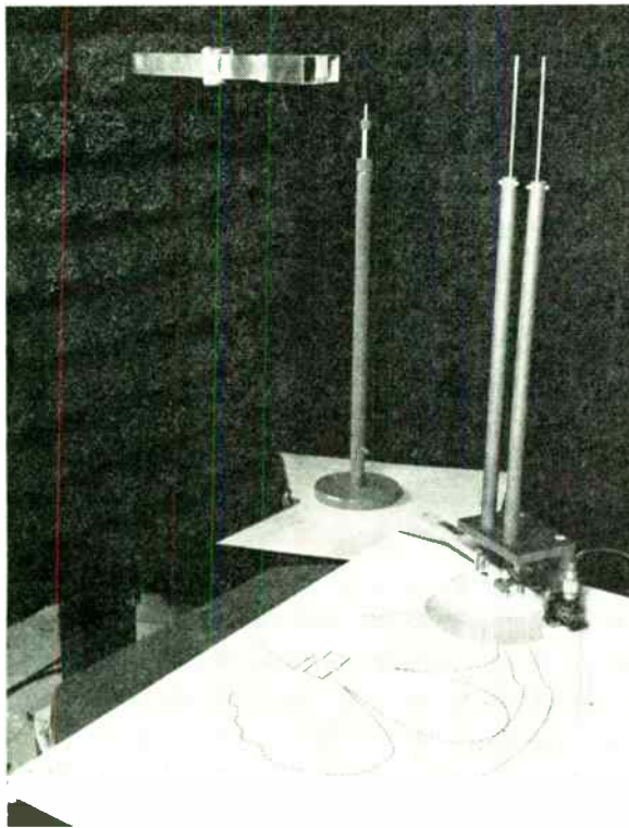
Fig. 1—Phase contour plotter in operation.
