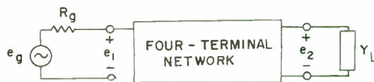
Fig. 1—Four-terminal network with variable load admittance and with generator having resistive internal impedance.
