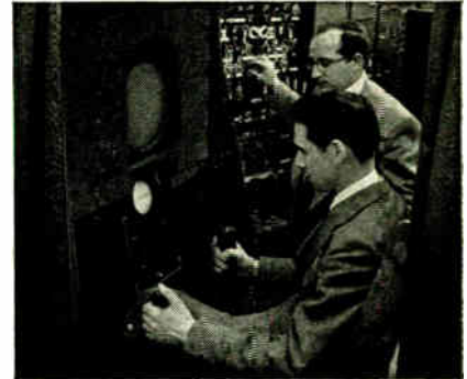
B. D. McVey (foreground) and E. Foxman examine operation of interceptor fire control system with equipment simulating in-flight performance of target, fire control system, and interceptor.
