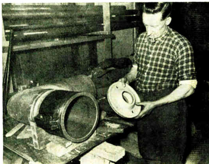
Fig. 14—90-degree mitered elbow- and spacer-insulator of 12-inch concentric line.
