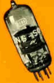
3CB6 (Prototype—6CB6) Heater Volts 3.15 Heater Current 0.6 A
