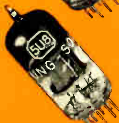
5U8 (Prototype—6U8) Heater Volts 4.7 Heater Current 0.6 A
