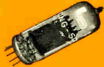
12BH7A (Prototype—12BH7) Heater Volts 6.3* Heater Current 0.6 A
