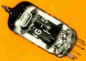
6AX7 (Prototype—12AX7) Heater Volts 3.15* Heater Current 0.6 A
