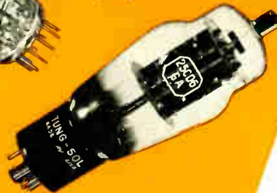
25CD6GA (Prototype—25CD6G) Heater Volts 25 Heater Current 0.6 A
