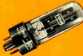
19AU4 (Prototype—6AU4GT) Heater Volts 18.9 Heater Current 0.6 A
