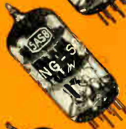
5AS8 (Prototype—6AS8) Heater Volts 4.7 Heater Current 0.6 A
