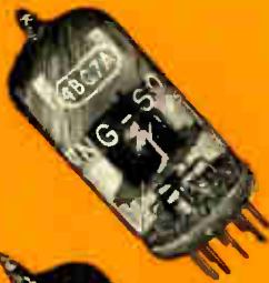
4BQ7A (Prototype—6BQ7A) Heater Volts 4.2 Heater Current 0.6 A
