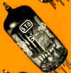
5T8 (Prototype—6T8) Heater Volts 4.7 Heater Current 0.6 A
