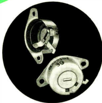
Latest "Humdinger" Series 39. Metal-case mounted with rivets or screws. Mounting surface serves as cover. Semi-fixed setting by screwdriver slipped into rotor slot —no shaft 2-watt 4 to 5000 ohms.
