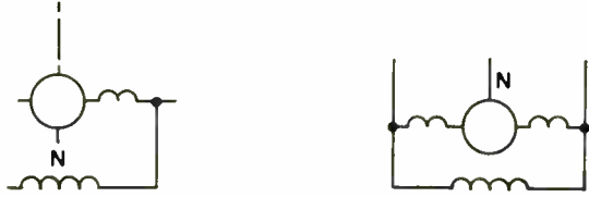
35.9.12 Direct-current 3-wire shunt generator with commutating and/or compensating field winding 1
