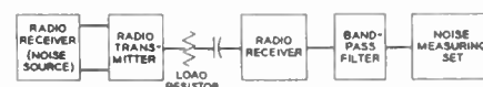
Fig. 5—Block diagram of circuit used in making the thermal noise loading tests.
