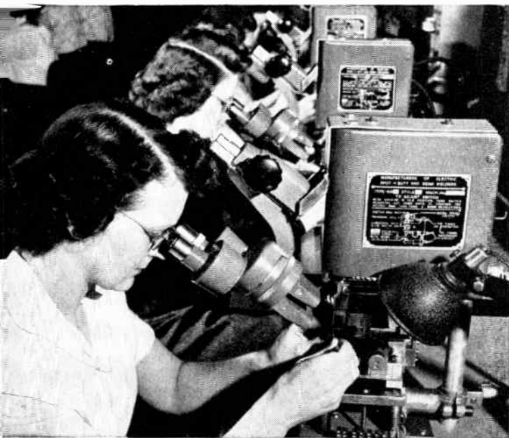
3. FORMING, SHEARING, AND WELDING WHISKERS on diode pin assembly calls for careful manipulation under microscope for accurately formed .003 inch diam. whisker.
