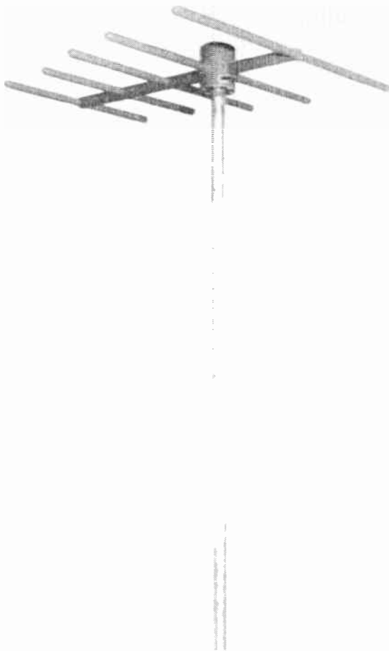
Fig. 5—Yagi antenna array used at terminal and repeater stations (Type 2488 A and B and 2489 A and B).
