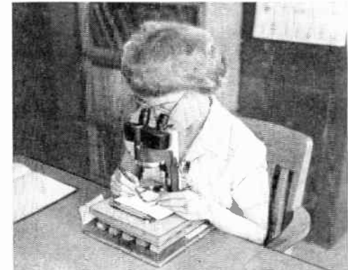
Microscopic examination studying surface conditions of cathodes.
