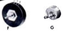
MODELS F AND G PRECISION SINGLE-TURN POTENTIOMETERS Feature both continuous and limited mechanical rotation, with maximum effective electrical rotation. Versatility of designs permit a wide variety of special features. F—3-5/16" dia., 5 watts, electrical rotation 359°—resistances 10 to 100,000 ohms. G—1-5/16" dia., 2 watts, electrical rotation 356°—resistances 5 to 20,000 ohms.
