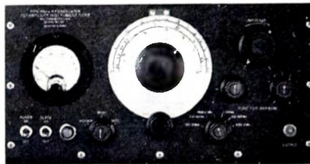
Type 320-A Phase Meter — frequency range 20 cycles to 100 kc.
