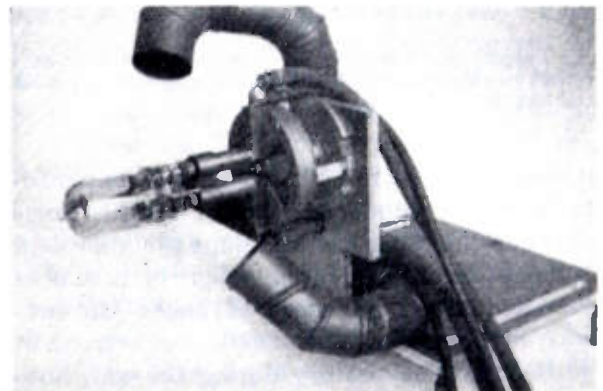
Fig. 3—Butterfly-tuned magnetron oscillator.
