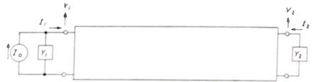
Fig. 39—Four-pole representation of an electron tube.
