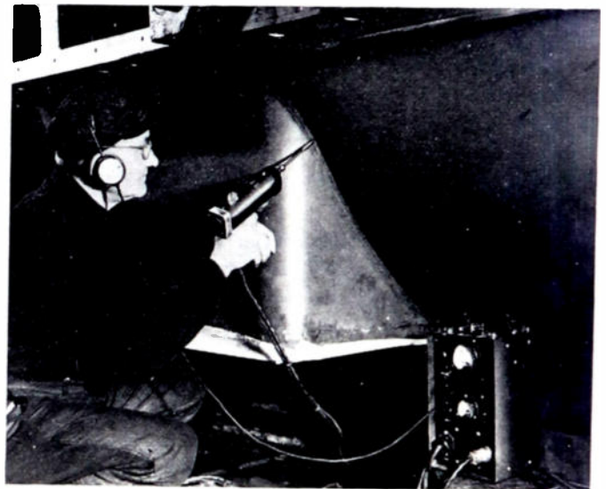
Fig. 10—Testing a seam weld for leaks on a large turbo-alternator casing.
