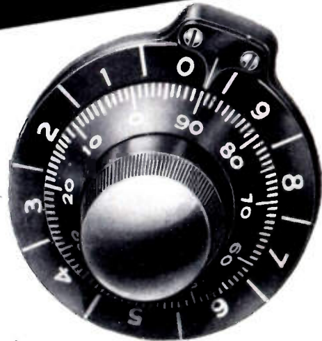
The inner, or Primary dial of the DUODIAL shows exact angular position of shaft during each revolution. The outer, or Secondary dial shows number of complete revolutions made by the Primary dial.
