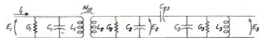
Fig. 12—Triple-tuned coupled circuit having both mutual-inductance and capacitance couplings in order to reduce effects of small asymmetries.
