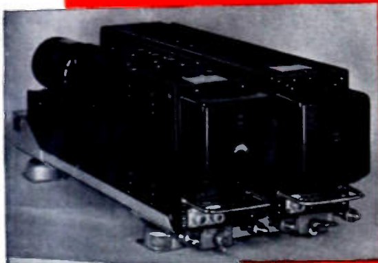
Collins 17L-2 vhf transmitter and 51R-2 vhf navigation-communication receiver in dual shock-mount.
