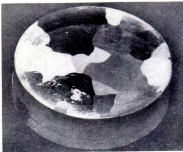
Fig. 13—Etch pattern of a rolled sample of AgCl. This crystal is unsuitable for conduction counting because of the large number of small crystals shown by the etch pattern. Diameter of crystal is 1\frac{1}{4} inches.
