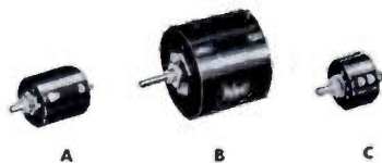
MODELS A, B, & C HELIPOTS A—10 turns, 46" coil, 1-13/16" dia., 5 watts—resistances from 10 to 300,000 ohms. B—15 turns, 140" coil, 3-5/16" dia., 10 watts—resistances from 50 to 500,000 ohms. C—3 turns, 13-1/2" coil, 1-13/16" dia., 3 watts—resistances from 5 to 50,000 ohms. — Ask for Bulletin 104 —
