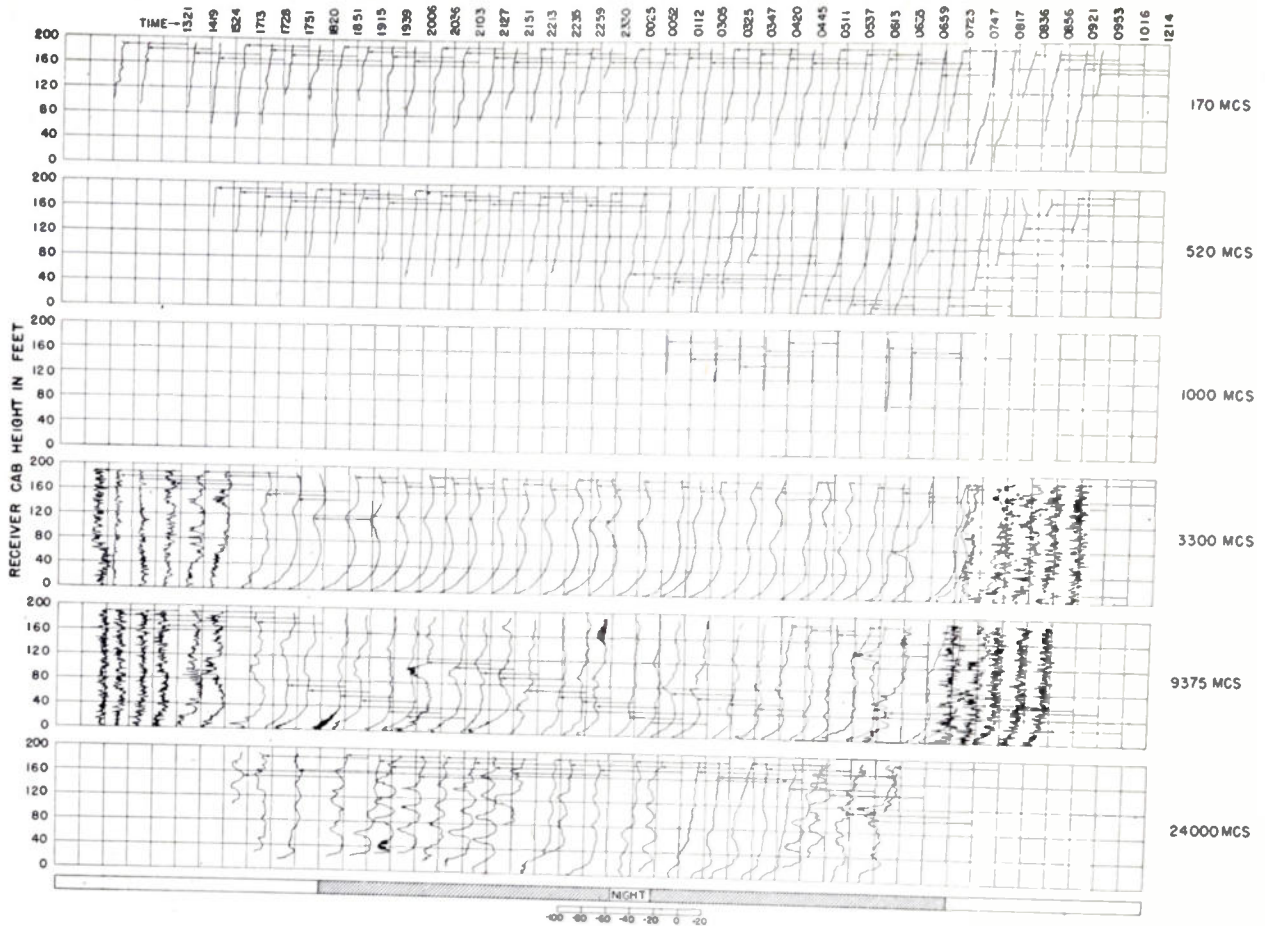
Fig. 8—A twenty-four hour cycle of received height-gain curves for the 46.3-mile path with transmitter cab at 1 foot. The time at which each curve was taken is indicated above the zero-db reference line for field strength. An arrow is drawn from each zero-db reference to the curve for which it applies. The field-strength scale in db, relative to the free-space field, is shown at the bottom of the figure.
