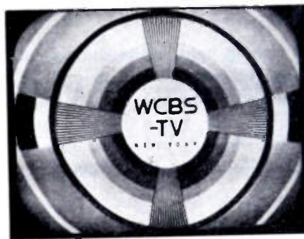
Fig. 10—Test pattern transmission over the two New York-Philadelphia television relay circuits connected in tandem.
