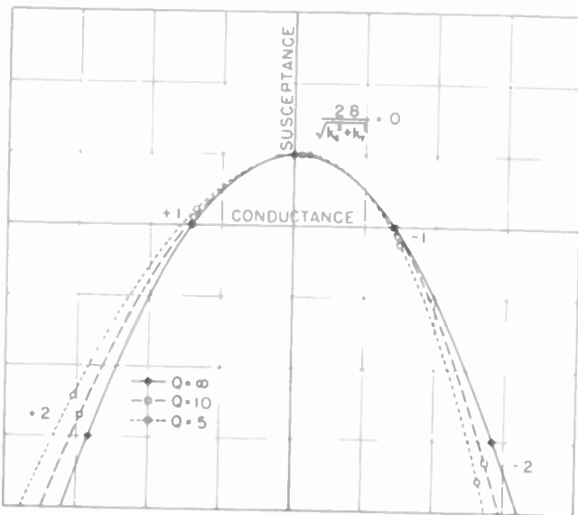
Fig. 3—Effect of Q on the normalized transfer admittance for two circuits of equal Q and identical tuning when the coupling is equal to the critical coupling. The ordinate scale represents unit values of normalized susceptance and conductance
