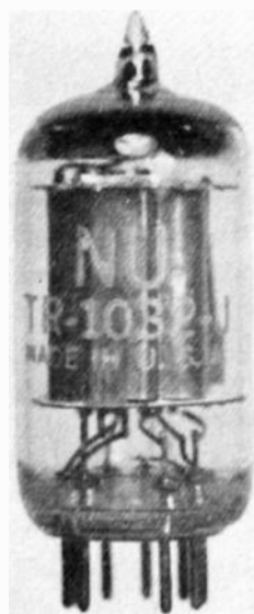
Fig. 3—Photograph of the miniature trigger tube.
