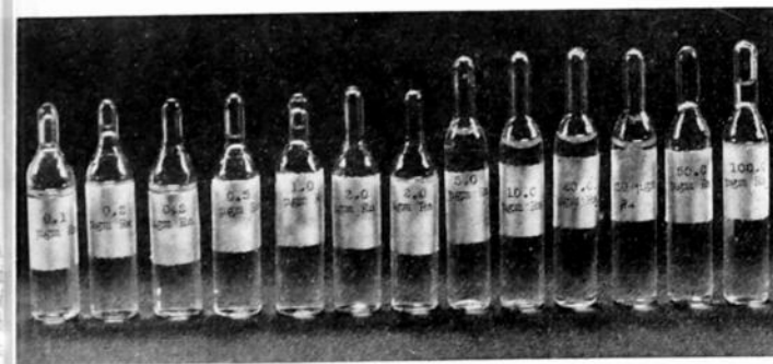
Fig. 4—Gamma-ray standards. Microgram standards of radium. The standards cover a range from 0.1 to 100 micrograms of radium, and are used for gamma-ray measurements of radium.
