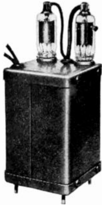
Above: Special DC power supply unit, input 115 volts 60 cycles—output 2500 volts filtered DC at 5 MA.
