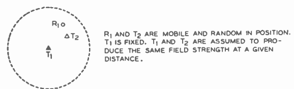
Fig. 2—Simple layout of vehicular system to illustrate interference at the mobile receiver.
