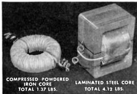
The laminated steel core coil requires about three times as much space as the newer powdered-iron core coil.
