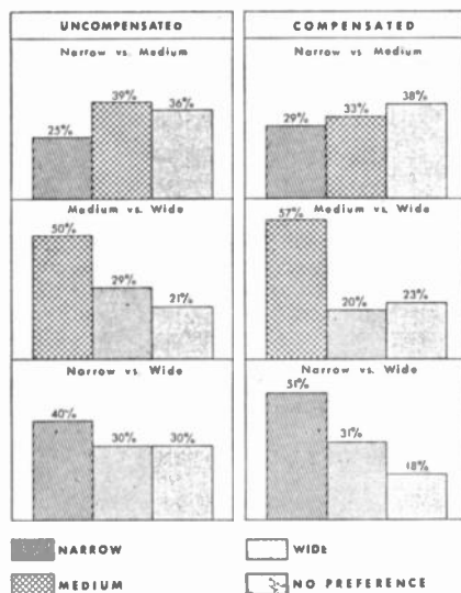
Fig. 3—The tonal-range preferences when listening to (a) uncompensated and (b) to compensated reproduction systems are shown by this chart. The listeners chose about the same bandwidth with either system; if anything, the majority prefer a slightly narrower range with a compensated than with the uncompensated system. This is probably explained by the fact that, with a compensated system, a somewhat wider range of frequencies can be heard than with an uncompensated system.
