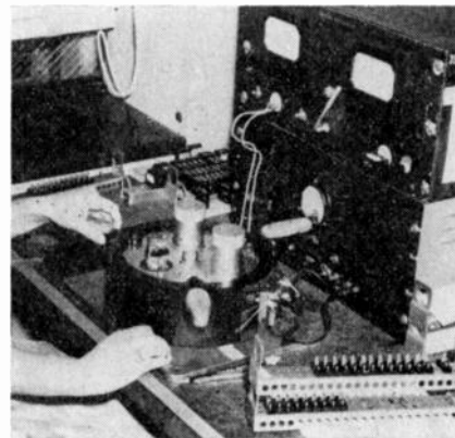
Fig. 8—Machine for final adjustment of plated crystal units by evaporation process.
