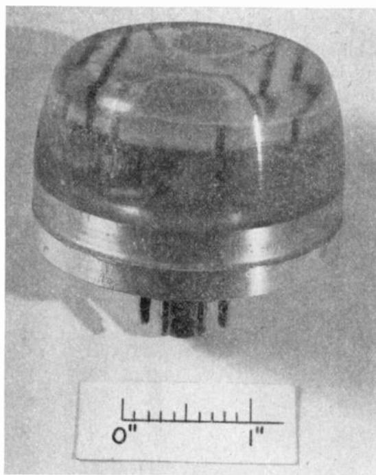
Fig. 49—Printed plug-in unit encased in NBS Casting Resin.
