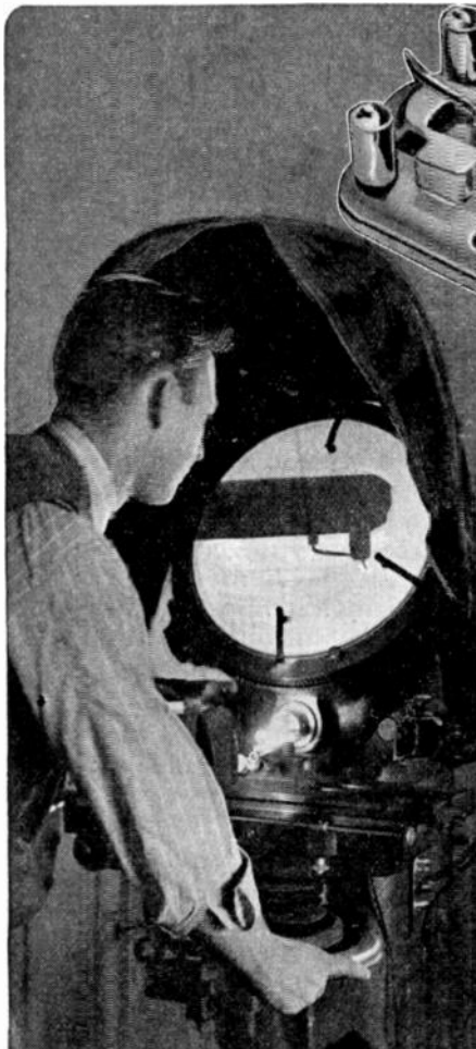
Comparator inspection of "Electro-Formed" precious Metal tip of replaceable "T" Type Needle used in the "LT" Cartridge.
