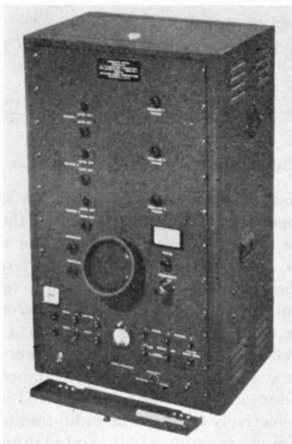
Fig. 8—Three-frequency impedance bridge, superheterodyne type.
