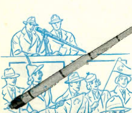
1937: The Western Electric "Machine Gun" mike does for sound pick-up what the telephoto lens does for photography. Sharply directional, this microphone makes sound "close-ups" of unusually long range.
