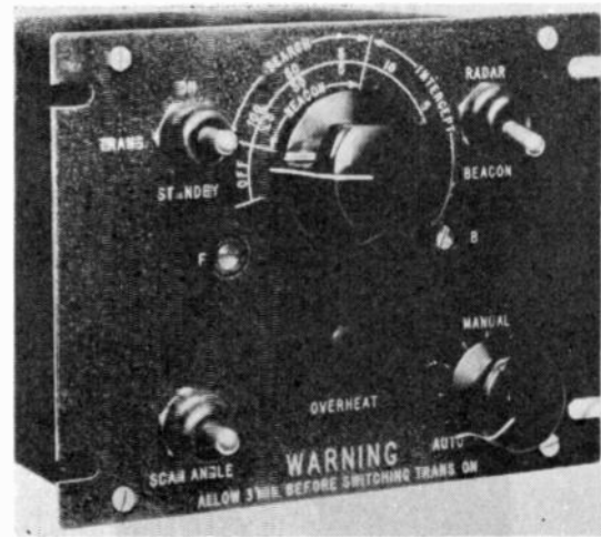
Fig. 47—Typical control box for pilot operation.
