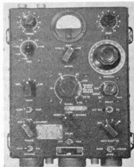
Fig. 30—Typical control box of modern aircraft search radar.
