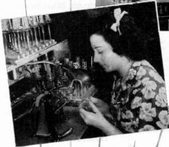
Assembling the electron gun
