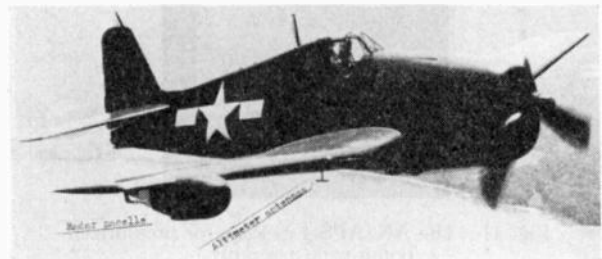
Fig. 42—Hellcat (F6F-3N) night fighter, showing AN/APS-6 wing radar nacelle and altimeter antennas.
