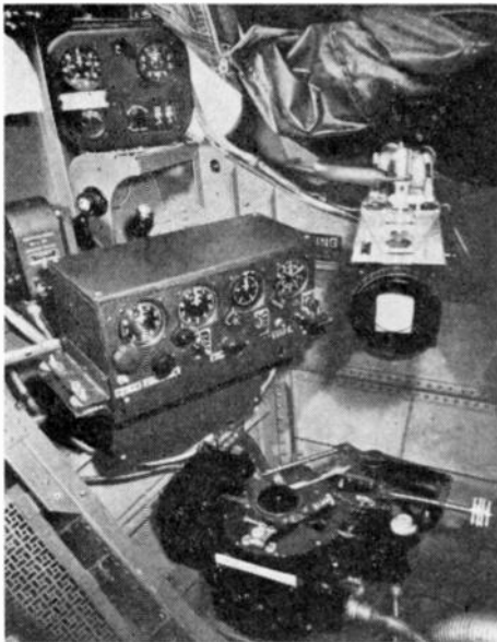
Fig. 52—Installation of synchronous-tracking-type bombing computer in Mariner (PBM-5) aircraft.
