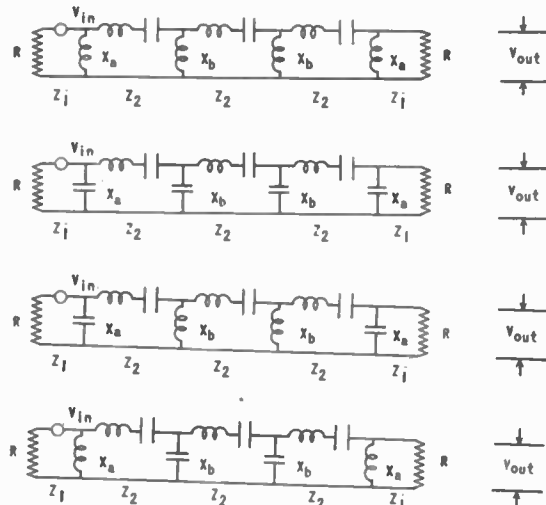
Fig. 10—Other resonant-circuit filters which may be analyzed by the method of this article.
