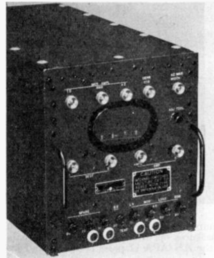
Fig. 21—Synchronizer of modern aircraft search radar.
