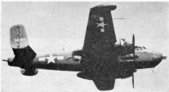
Fig. 13—AN/APS-3 wing-tip radar nacelle installation in Mitchell (PBJ).
