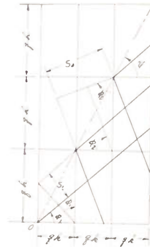
Fig. 4—Geometry of the wire spacing. Progressive layering.
