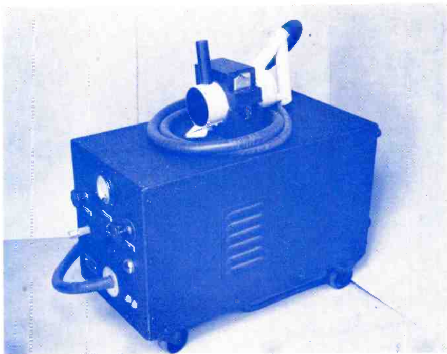
ELECTRONIC RIVET DETONATOR HIGH-FREQUENCY HEATING OF EXPLOSIVE RIVETS MODERNIZES AN OLD ART
