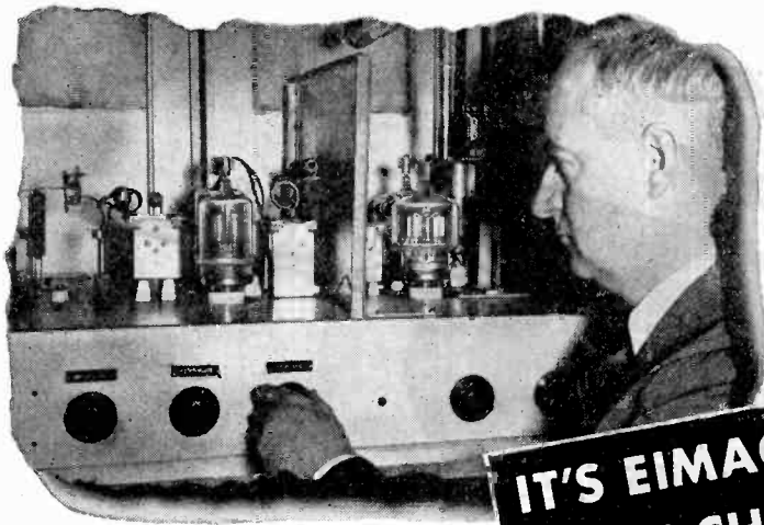
A. H. Brolly . . . Chief Engineer of Television Station WBKB, Chicago, adjusts the grid circuit of the Eimac 304-TL's in the Class B linear stage of the video transmitter.
