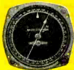
MN-37 Automatic Compass Bearing Indicator
