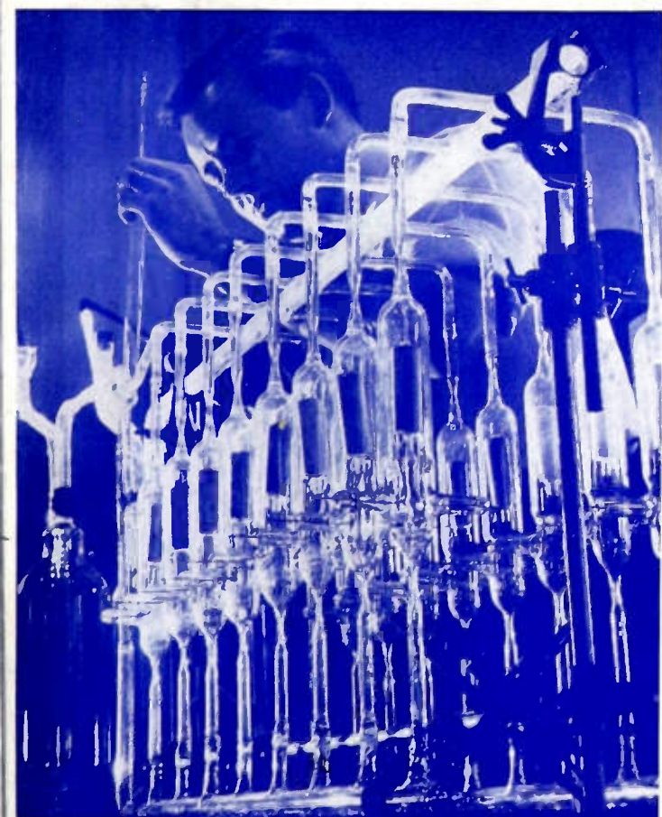
TEST OF PAPER CAPACITORS IN VACUUM (At -300^{\circ} F to +250^{\circ} F)
