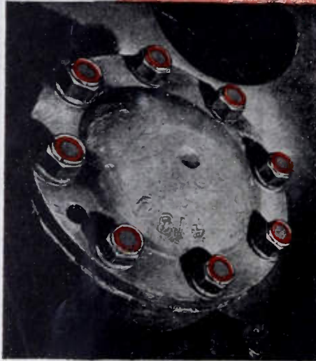
These Elastic Stop Nuts are holding the driving flange. Even with frequent starts and stops, and the steady use the wheels of an express truck get, these nuts hold fast.
