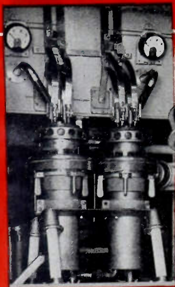
A pair of water-cooled RCA-9C21's in a 100-KW, 25 megacycle, r-f heating oscillator.
