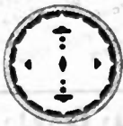
16-point TUNG-SOL disc permits good support under all conditions.
