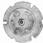
Motor blower for circulating air within radio transmitter, for tropical service.
