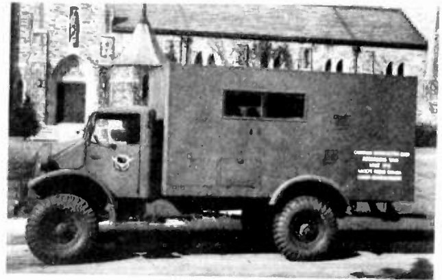
Fig. 7—The van which is used by the CBC correspondents in England for remote and recording work.
