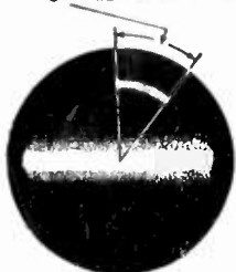
Oscillogram of the operation of a two-way snap-switch, accurately timed in milliseconds. The segment represented by the curved trace or arc, measures 39°, or the equivalent of 1.8 millisecond.
