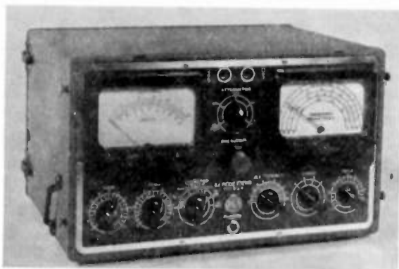
Fig. 6—RCA Type 312A radio-noise meter showing control panel.
