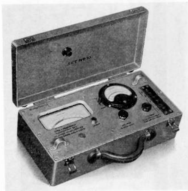
Fig. 13—Photograph of thermocouple set.
