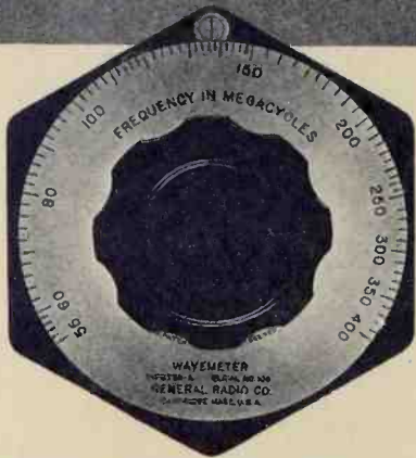
Direct-reading dial calibrated from 55 to 400 Mc, with open scale. Six-sided end plates for resting wavemeter horizontally in a number of positions
