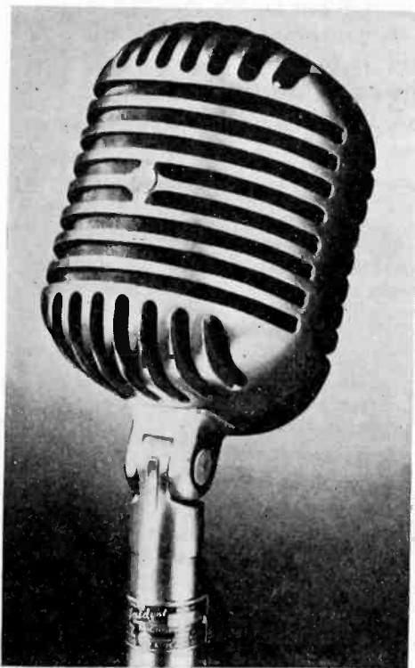
An acoustical phase-shifting network is responsible for the unidirectional characteristic of this dynamic microphone
