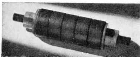
Five sections of a powdered-iron core assembled on a threaded rod of insulating material
