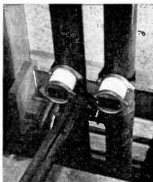
Fig. 11—Lower end of oscillator plate tank circuit, showing the blocking condensers feeding the load.
