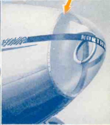
BUILT-IN DIRECTION FINDER Mounted behind non-metallic nose —Reduces drag—Eliminates icing.
