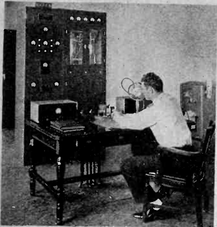
WESTERN ELECTRIC ultra high frequency Police Radio Transmitter, Station W2XEM, Newark, N. J.
