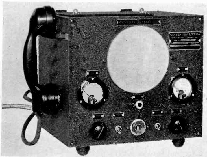
Fig. 17—Rectifier and control unit model 4MR1A1 for 15-watt 30- to 42-megacycle transmitter and receiver used in two-way police radiotelephone communication system.
