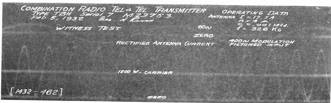
Fig. 8—Oscillogram of rectified antenna current.
