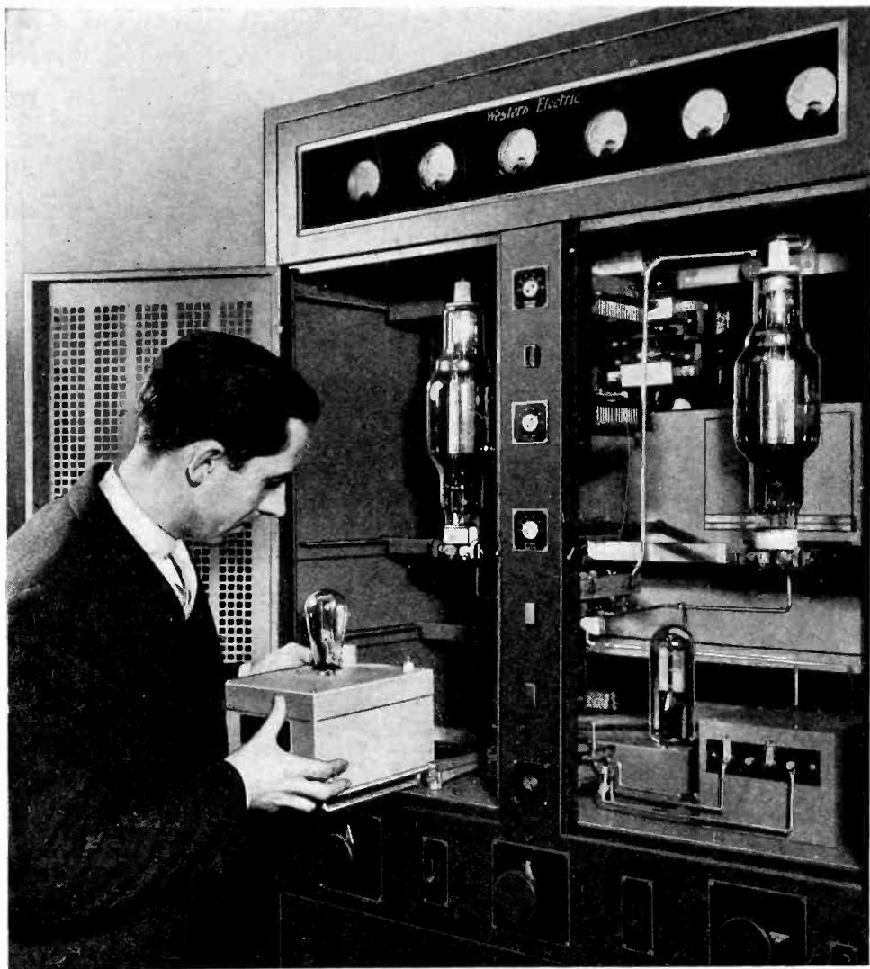
Fig. 5—Placing crystal oscillator unit in the transmitter.
