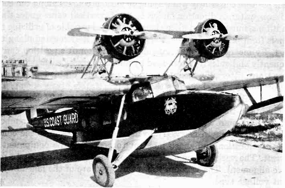
Fig. 30—Model CGR-19-B direction finder loop mounted on U. S. Coast Guard amphibian plane.
