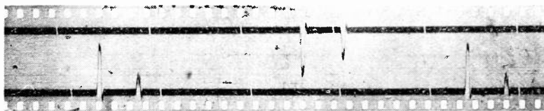
Fig. 6—Note predominant 565-km virtual height. Note, however, faint evidence lower layer in upper trace. (4045 kc, 3:50 P.M., E.S.T., August 13, 1930).
