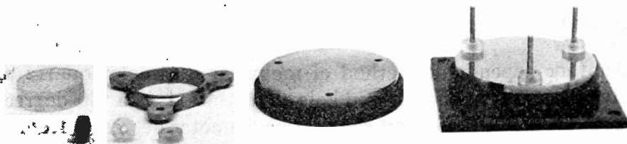
Fig. 7(a and b)—Mounting for cylindrical quartz plate (assembled and disassembled).
