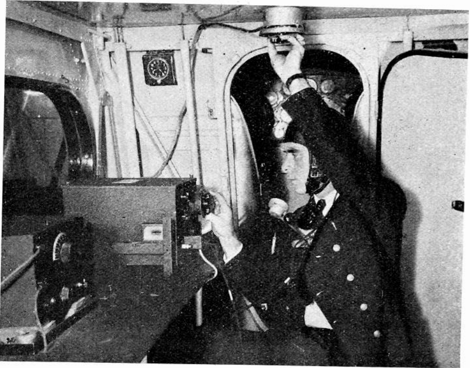
Fig. 32—Interior arrangement of Model CGR-19-B radio direction finder installed on U. S. Coast Guard plane.
