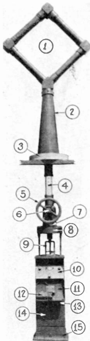
Fig. 17—U. S. Coast Guard radio direction finder, Type-A, Model CGR-17-C.
