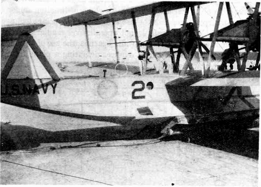
Fig. 29—U. S. Coast Guard Model CGR-19-B, radio direction finder loop mounted on U. S. Navy PN-12 seaplane.
