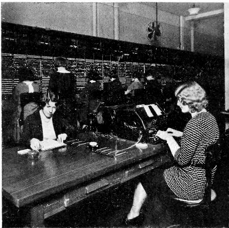
Fig. 2—Transatlantic telephone operator's position showing arrangement of printing telegraph equipment.
