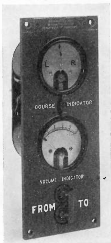
Fig. 12—Course and volume indicating instruments with reversing switch for use with reed converter on a red, brown, or yellow radio beacon course.
