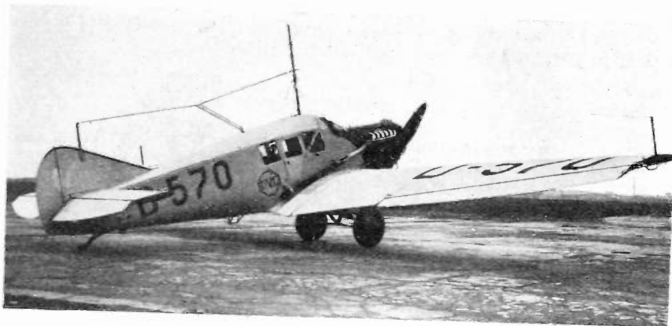
Fig. 9—Airplane for measurements (longitudinal dipole shown by heavy lines).
