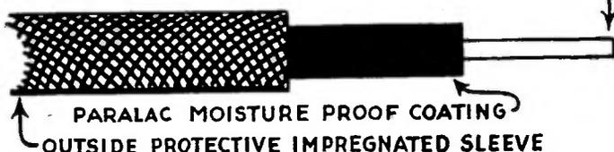
The Paralac coating is applied between the copper conductor and the outer sleeve, insuring moisture protection and adding greatly to the voltage breakdown. In use, the Paralac coating and outer sleeve push back together without bunching.
