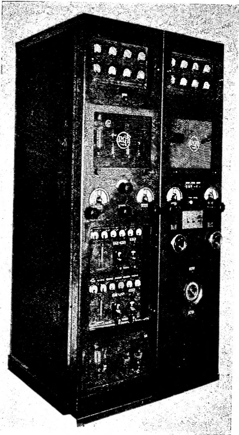
Fig. 9—One-kw broadcast transmitter. Left front view.
