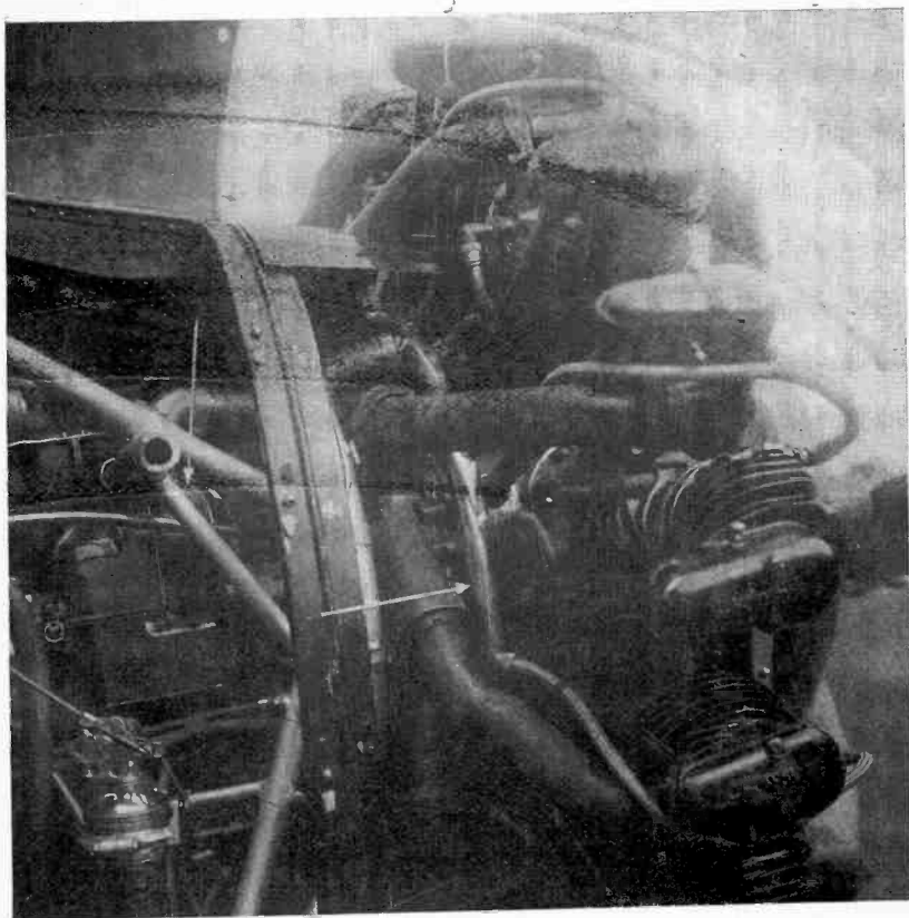
Fig. 20—Installation of the commercial type shielding assembly on Bureau's Wright J-6 airplane engine.
