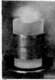
Fig. 5—186 kc, mounting B , height 38.3 mm, dia. 24.715 mm.
