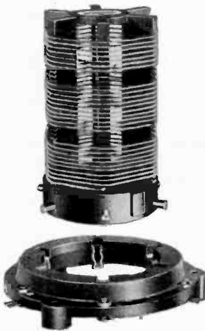
Illustrates the REL one-piece bakelite plug-in coil and base—space wound—heavy enamel covered wire—positive base contact.
