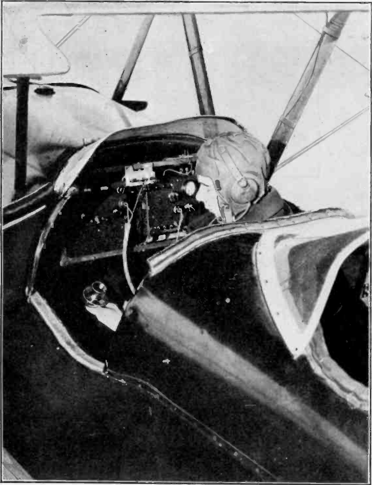
Fig. 33—Burgess Radio Equipment Installed in Travel Airplane.
