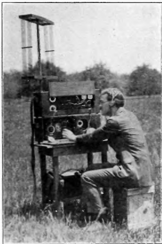
FIGURE 4—Field Strength Measuring Set in Operating Condition in the Field
