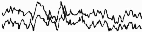
FIGURE 36A—WJAC, Boston, Massachusetts, received at Newton Centre, Massachusetts, 11 kilometers (7 miles) distant, November 13, 1923, on antennas 30 meters (97 feet) apart on centers. Upper record on large open antenna by Shaw; lower record on small open antenna by Pickard. Record is 4 minutes and 40 seconds long
