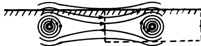
FIGURE 9—Distribution of Magnetic Lines About the Buried Wires Wires and current flow are perpendicular to the plane at the paper
